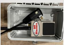
**4)** Secure the lid to the lockout tagout box and lock accordingly.
